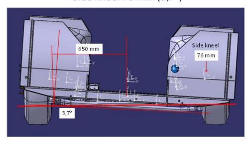
Low rotation in z-dir - estimated on the ground and 650 mm to the side in y-dir.
