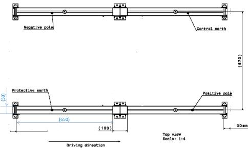
**3** Top View of conductive rails on roof with dimensions
