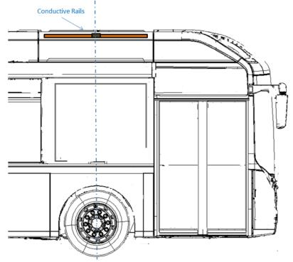
2 Side View of bus roof front section highlighting conductive rails
