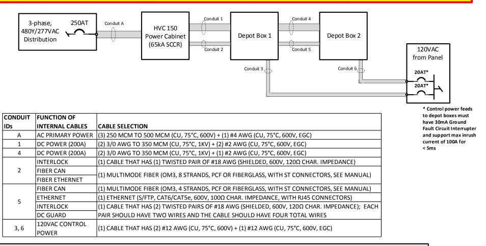
N1. Equipment enclosures must be externally labeled according to local codes by the installing contractor to notify service personnel to verify absence of voltage from more than one power source.
