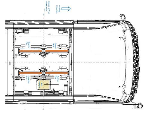
Figure 6. OPPCharge Capable Conductive Rails Installed on the Top of Electric Buses<sup>1</sup>
