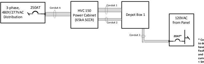
\* Control power feeds to depot boxes must have 30mA Ground Fault Circuit Interrupter and sup port max inrush current of 100A for < 5ms
